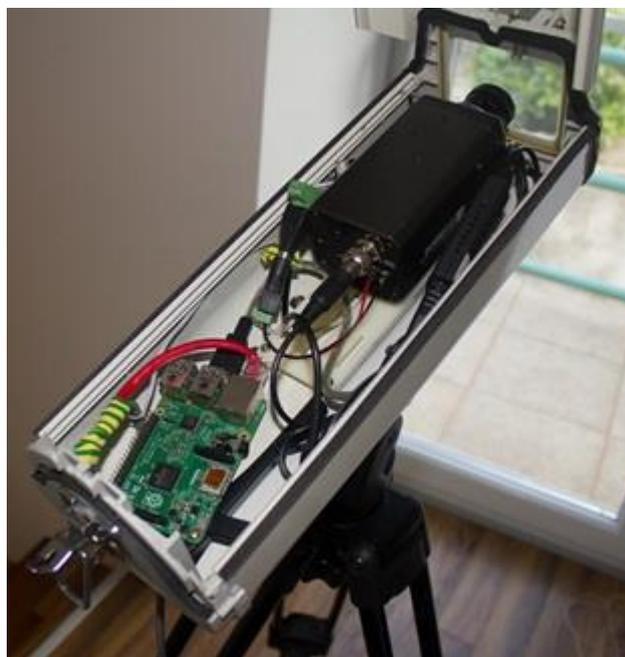
Figure 5 – Assembled prototype with all components contained within a standard video camera housing.
